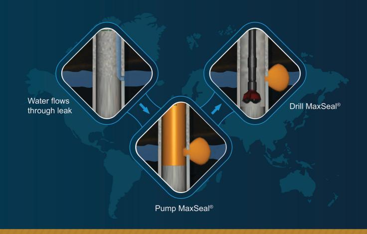
Long-term zonal isolation issues with oilfield cement annuli commonly result from cyclic temperature and pressure loading during the lifetime of the well. Cement mechanical properties such as brittleness and low tensile strength affect the long-term durability of the cement seal.
